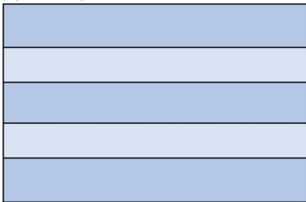
Fig. 10 Schematic representation of grain boundaries in a polycrystalline materials and b multilayered heterostructures. Variations in colors represent different crystallographic orientations in grains or different material compositions in solid solutions or heterostructures. Grain boundaries are denoted with black lines
